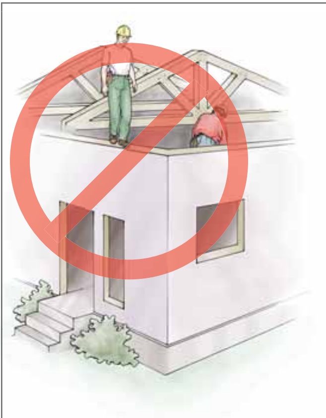
Workers must not walk on top plates of walls.
