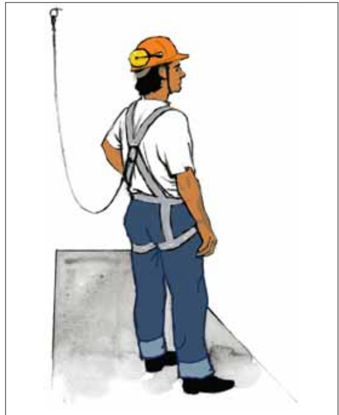
This is an example of a fall arrest system.
