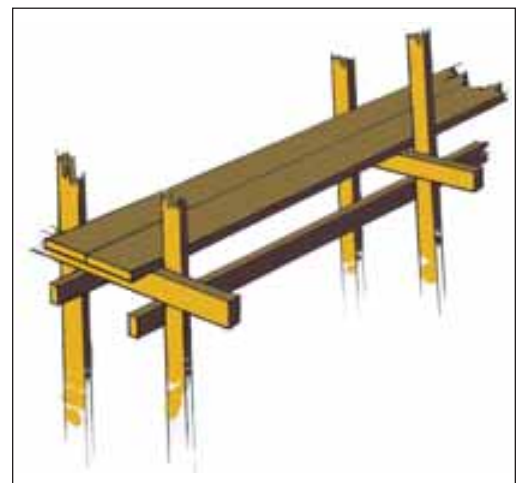
Example of planks placed side by side.
