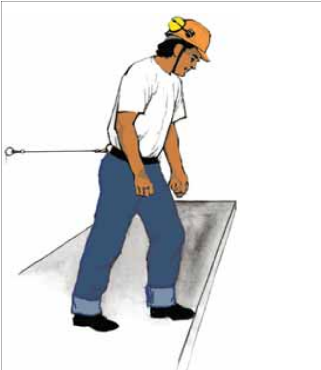
This is an example of a fall restraint system where worker cannot fall off edge.
